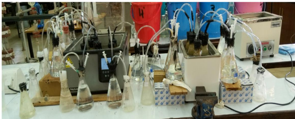
Figure 2 Biogas production setup (Adopted from Catherine and Twizerimana, 2022)
