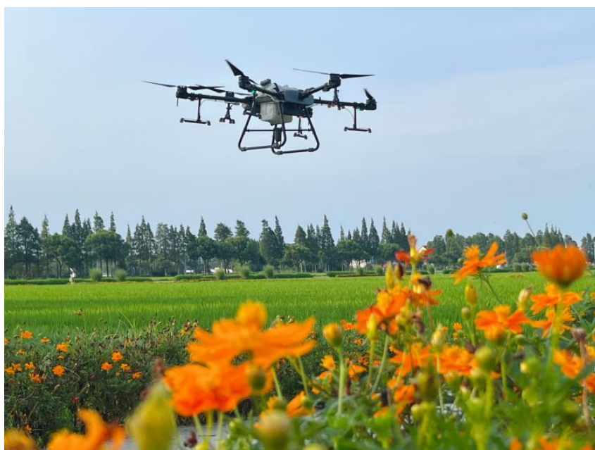
Figure 4 A drone (UAV) conducting remote sensing over a rice field to monitor crop nitrogen status in real time (Photo from Zhigang Fu)
